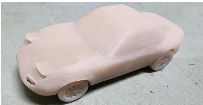
This Mazda Miata was created using the Blender 3D modelling software and then printed using the school's Resin 3D printer.
